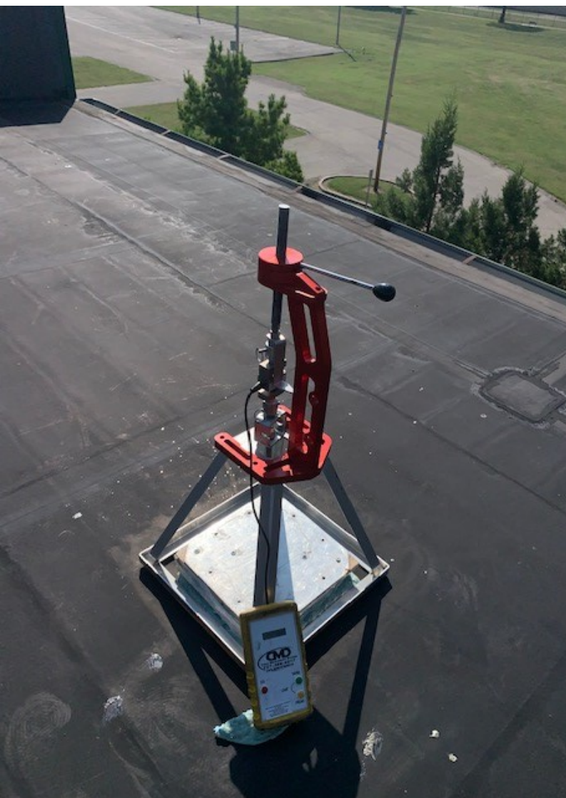
TEST AREA #3, 12" BEAD SPACING, 230 PSF, FAILURE MODE WAS INSULATION FACER AND ADHESION FROM BOTTOM FACER. ATTACHMENT TO EPDM WAS STABLE.
