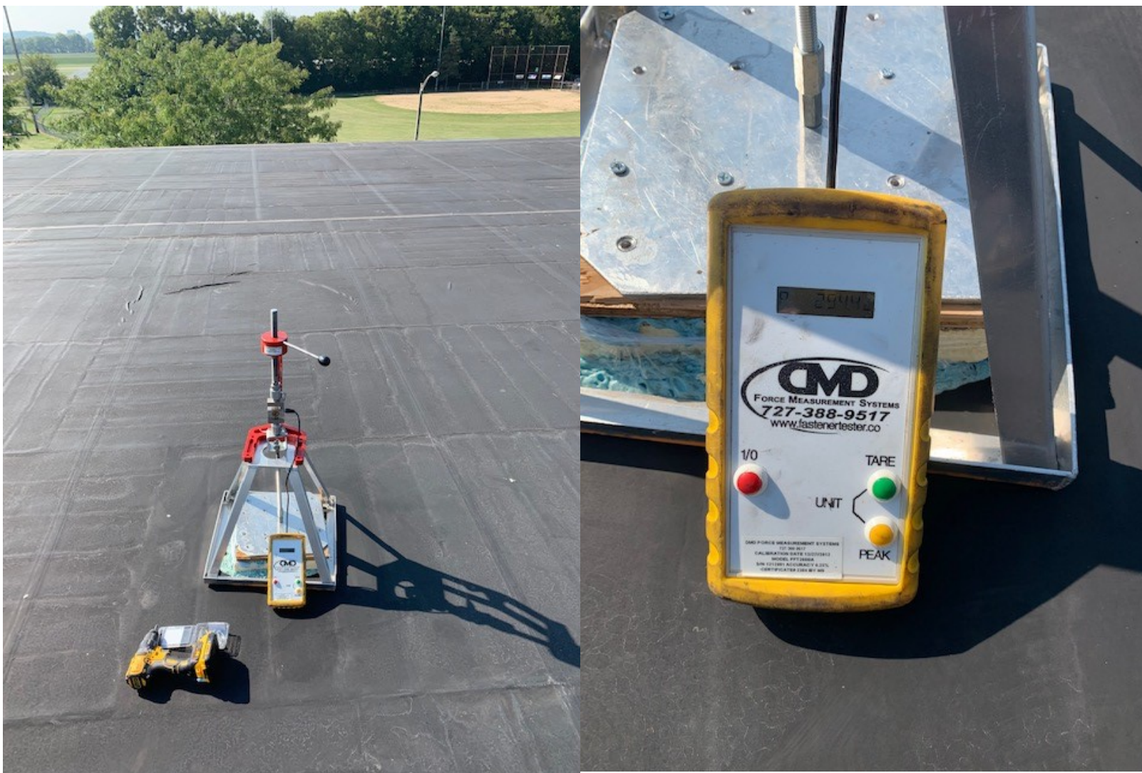
PULL TEST #2, 6" BEAD SPACING, 294 PSF, FAILURE MODE WAS INSULATION FACER
