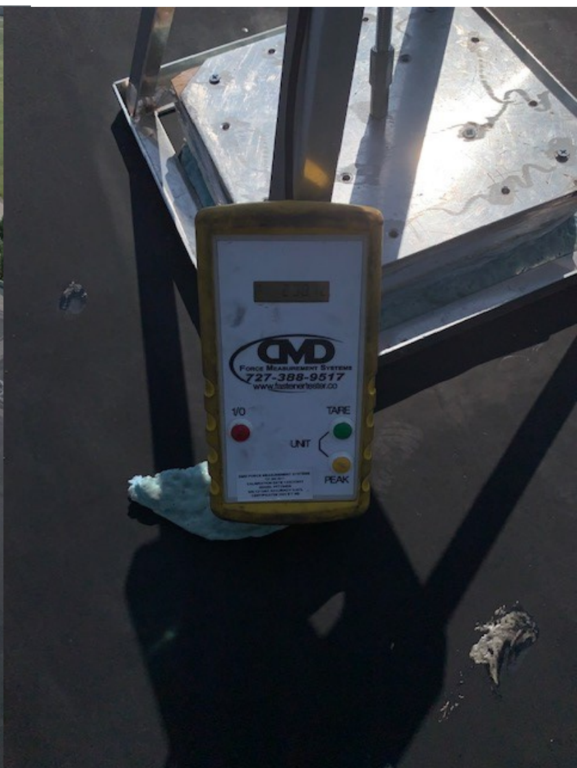
TEST AREA #3, 12" BEAD SPACING, 230 PSF, FAILURE MODE WAS INSULATION FACER AND ADHESION FROM BOTTOM FACER. ATTACHMENT TO EPDM WAS STABLE.
